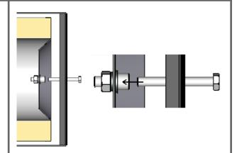
Screw the fixing screw tight.
